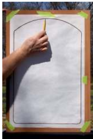
Cut Paper Larger Than Opening. Tape To Routed Side And Make Rubbing With Edge Of Pencil Lead .
