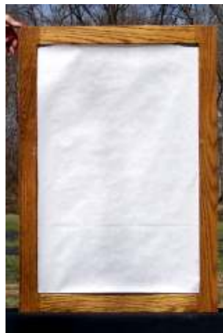
Cut Paper To Fit Inside Routed Area, Minus 1/8" to 1/4" To Assure Fit OF Glass.
